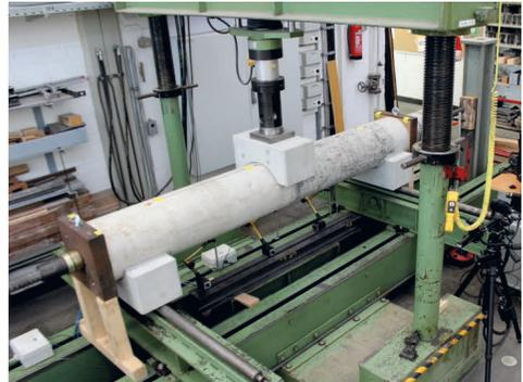
Hollow concrete members with a wall thickness to diameter ratio of  $t/D = 1/10$  were used in all tests. The micro-reinforcement ( $\varnothing 1$  mm, mesh size 20 mm) was dimensioned using the previously described approach to determine the minimum reinforcement (cf. section 4.3.1). In addition to a variation of the load position and thus of the shear slenderness  $a/d$ , a normal force  $N$  was applied in two tests (Table 5).
