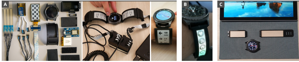
Fig. 5.5.: Our research platform currently involves two StrapDisplays (a+b) and a tablet prototype (c). The (a) e-ink displays are paired with touch sensors and put into a housing and connected to the required controllers. The (b) OLED watchstrap is assembled in a similar way. The (c) tablet prototype consists of a stencil cover placed on the full-color displays of a tablet.
