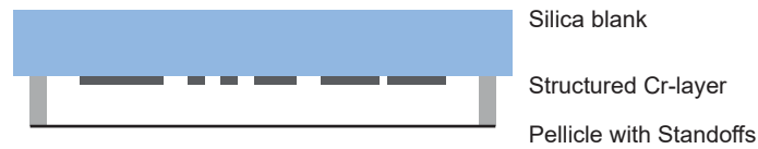
Figure 1.2: Model layout of a typical photolithography reticle.
