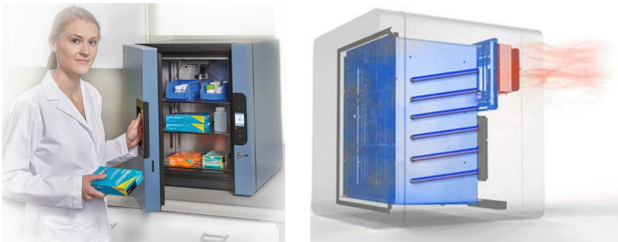
Figure 30. Commercial use of solid state thermoelectric devices. The figure on the left shows a typical application for this product, while the figure on the right shows the operation principle of the device, whereas a refrigerant that absorbs and transfer heat away from the refrigerator chamber is used. This heat is then dissipated into the environment by a macro-sized thermoelectric module that functions as a heat pump. Courtesy of Helmer Scientific Inc [48].
