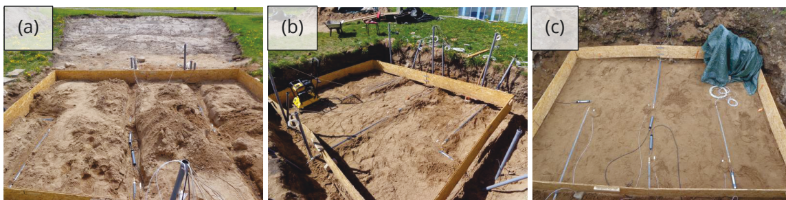
Figure 4.5. Installation of measuring devices (tensiometers, water content, temperature and electrical conductivity) in (a) Layer 1, (b) Layer 2, and (c) Layer 3
