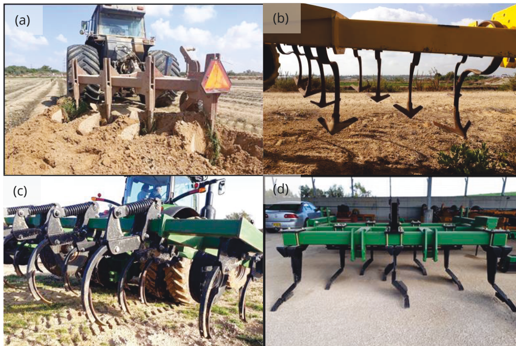
Figure 2.10. Tillage tools used for recovery of the infiltration rate in SAT recharge basins: (a) Plow (b) Sweep-knives (SK) Cultivator; (c) Chisel-knives (CK) cultivator and (d) Subsoiler (paraplow type). Source: Negev et al. (2019)
