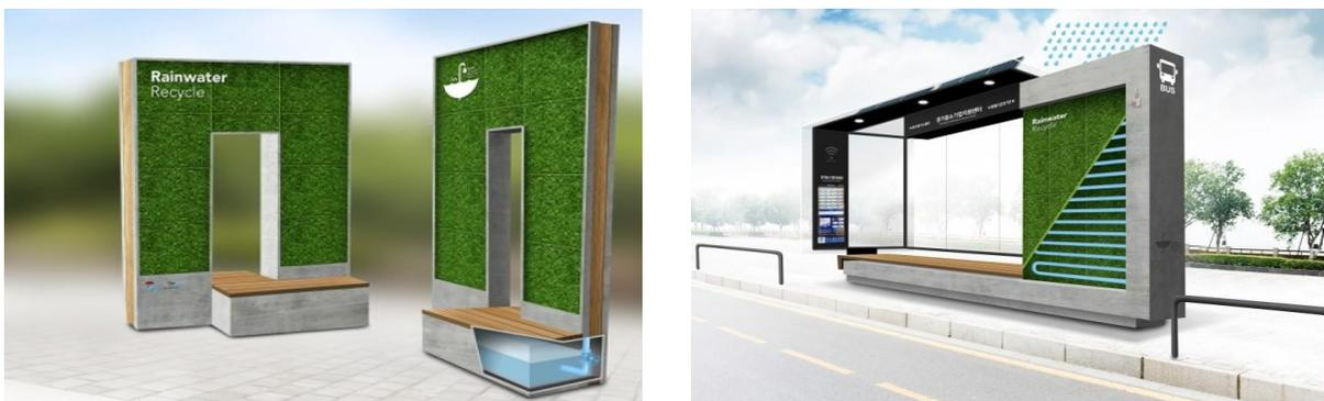
**Figure 7.24** City Tree design using rainwater (left) and its application (Smart Eco Station; right) (Source: SG, 2018)
