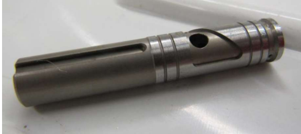
Figure 11: “Like new” helical groove actuator piston after first disassembling after 1 Mill. Cycles
