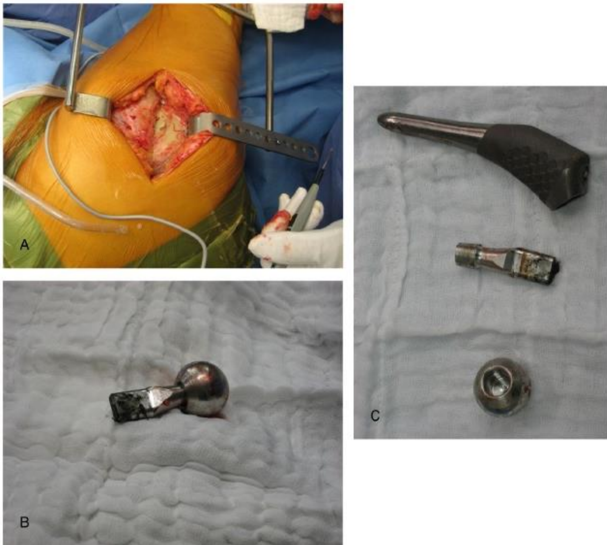
Figure 3. (A) Revision surgery of a hip joint with soft tissue reaction to metal ions around the implant. (B) Photograph shows the base of the modular neck with severe wear and (C) parts of a hip prosthesis with severe signs of wear at the base of modular neck (Vundelinckx et al., 2013).
