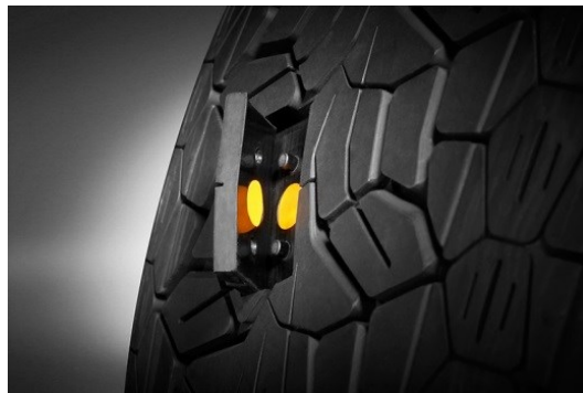
Figure 8.1: Sensor embedded in tire-tread to detect tire pressure and sense road conditions [181]. Reproduced from Continental Tires – Press release August 12, 2017.
