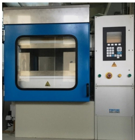
Figure 3.7: Heated press utilized to prepare the samples
