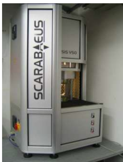
Figure 3.8: A view of the utilized rubber process analyzer
