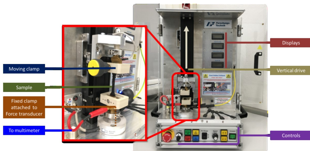
Figure 3.10: In-house built piezoresistance measurement device with a magnified view of the sample clamps (left)
