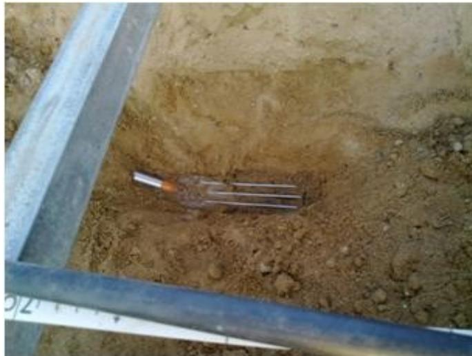
Fig. 5 TDR probe and a pF-Meter next to each other as one sensor pair.
