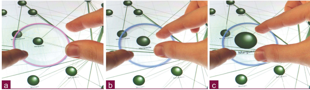
Fig. 4.6.: Using the continuous gesture, the user can switch from Local Edge (red) to fisheye (blue) function and continuously set the magnification factor as its primary parameter.
