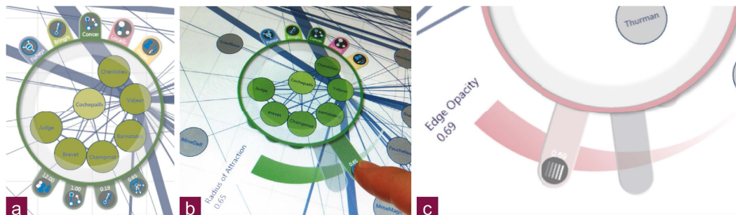
Fig. 4.3.: The lens provides an upper menu for selection of lens functions and handles at the bottom for parameter adjustment which are encoded with the associated lens function color (a). A slider around the lens can be invoked for parameter adjustment (b-c).
