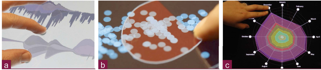
Fig. 2.5.: There have been various solutions adapting touch interaction to information visualization techniques, e.g., stacked graphs (a, TouchWave [BLC12]), scatter plots (b, [SS14]), and star plots (c, [Lan+15]).
