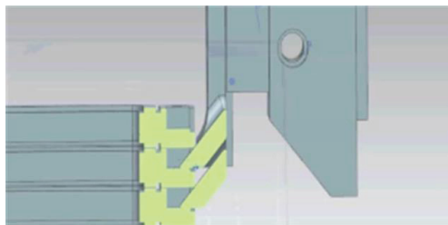
Figure 7: Movement of the clamp fingers
