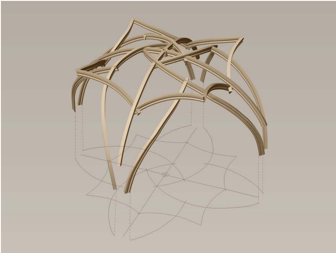
Fig. 3: CAD model of the spatial system of the ribs, showing only the profiled parts (CAD M. Aranda Alonso)
