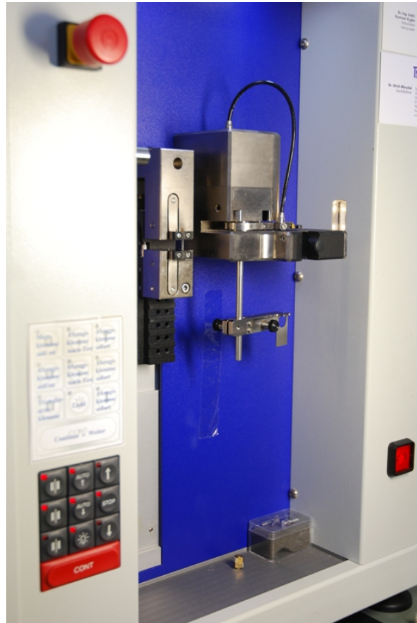
Figure 3.3: The picture of the tensile test device for single filament: FAVIGRAPH semiautomatic equipment
