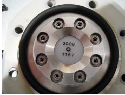
Figure 3.8: PTB radioactive source on a Ta backing installed in the target holder for efficiency calibration.
