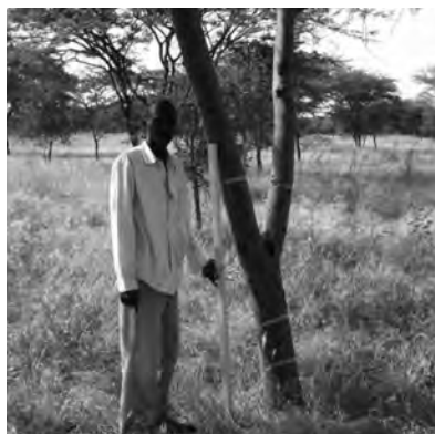
Figure 3.9 Measuring pole used for marking the position of tree diameters
